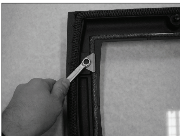
Fig. 11. Tightening The Glass Clip
