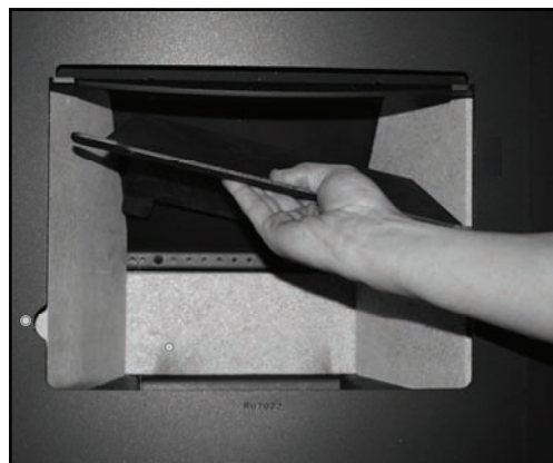
Fig. 4. Inserting The Throat Plate
