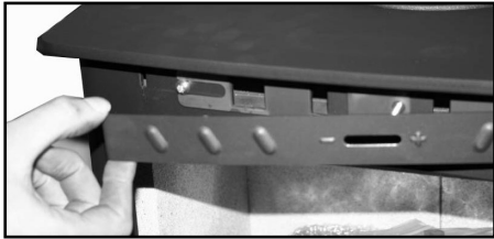
Fig. 4b Lifting cover from body of stove
