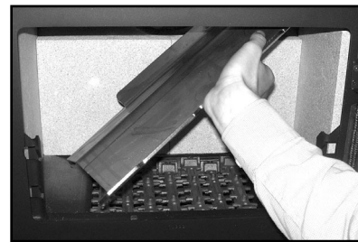
Fig. 13 Inserting Throat Plate in to Sherborne Medium Multifuel.
