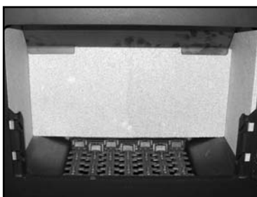
Fig. 3 Liners, throat plate and grate in the Acorn.
